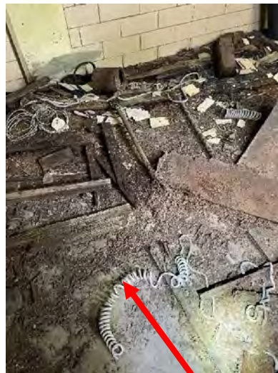
Photo 24: Asbestos-Containing Rope Gasket Material
